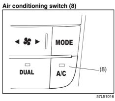
The air conditioning switch (8) is used to turn on and off the air conditioning system. To turn on the air conditioning system, push in the switch; "A/C" will appear on the display and the indicator on the switch will come on. To turn off the air conditioning system, push in the switch again; "A/C" and the indicator will go off.
